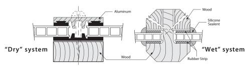
Figure 10. Description of Typical Two-Part Wood Connecting Profiles Currently used in the Market
