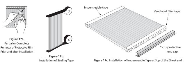
on Open Ends of Sheet Installation of Ventilated Tape at the Bottom of the Sheet
